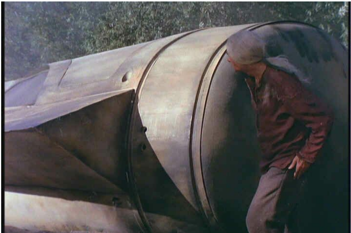
Photo 20: closed gull wing and heat shield about 6 feet diameter and 2 feet deep, cleaned for the TV episode, 1974, https://www.goingfaster.com/icarus/virdonopening.html
