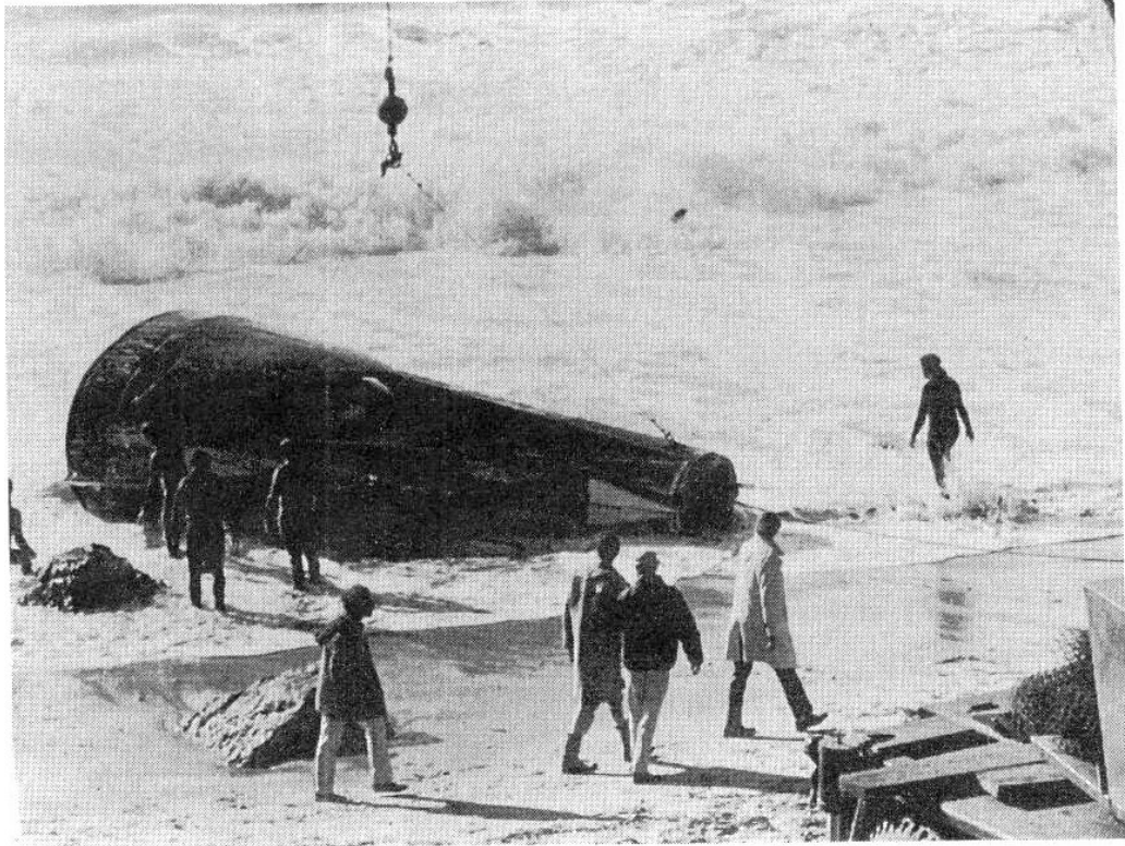
The spacecraft was damaged when it broke free from its cables and crashed into the rocks.
