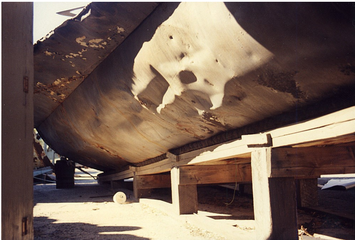
Photo 18: Phil Broad, 1973-74, the underside showing rock damage.
