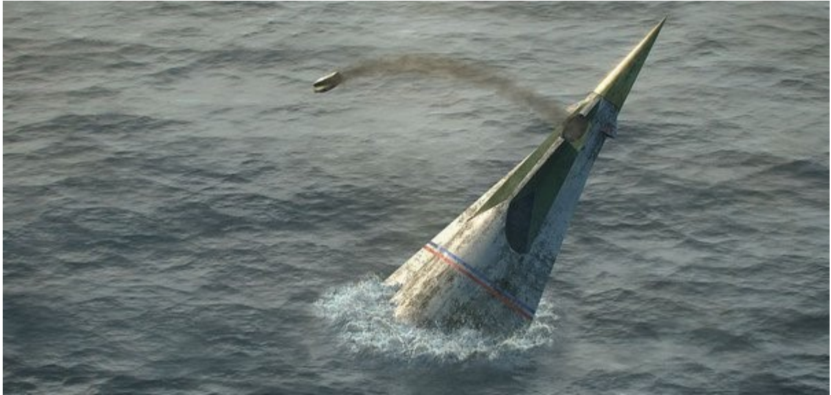
Photo 2: The escape hatch cover blows off after splashdown.
